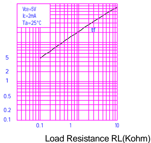
Fig.11 Response Time vs. Load Resistance
